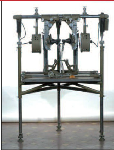
Fig. 10 – The transportable Stereosimplex stereo-plotting instrument, which was based on optical-mechanical projection, was designed by Santoni and built by Officine Galileo. (Source: IGMI Museum)
